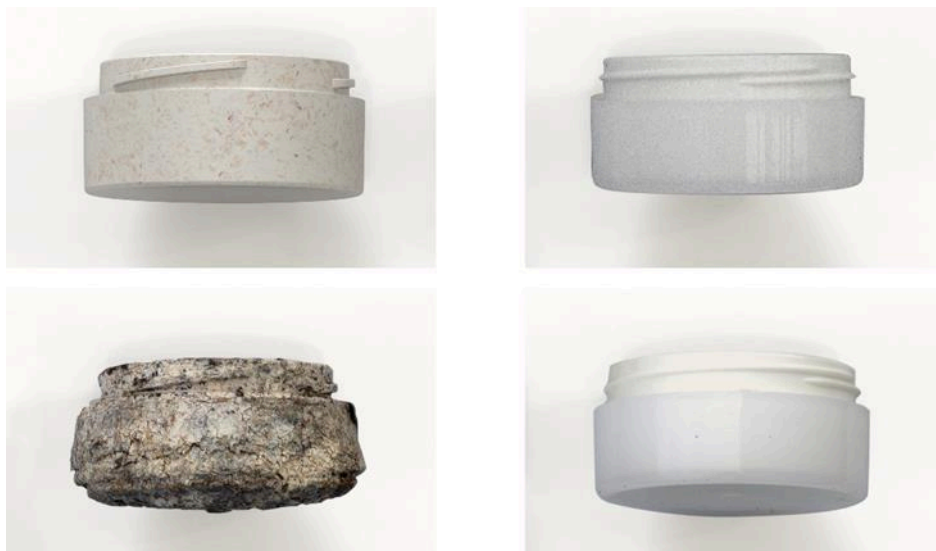
Figure 1. Sulapac Premium (left) and polypropylene (right) jar before composting and after being held in an industrial compost for 21 days (EN 13432).
